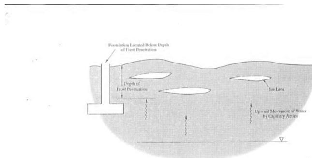
**Figure 18.2.** Formation of ice lenses. Water is drawn up by capillary action and freezes when it reaches the frozen soil, which is located within the depth of frost penetration. The frozen water forms ice lenses that cause heaving at the ground surface. Foundations placed below the depth for frost penetration are not subject to heaving.
